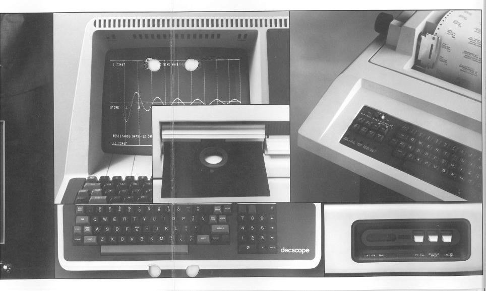
extremely easy to use. It features many practical, functional and operator-oriented innovations, including 30-characters-persecond throughput, quiet operation, varial forms width, and multi-part forms capability. The typewriter-like keyboard assures easy user adaptation.
