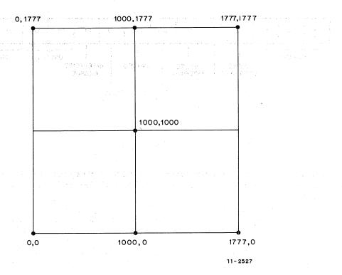
Figure 4-6 Scope Grid Coordinates X, Y
