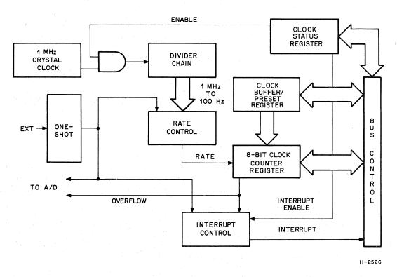
Figure 3-1 Clock Block Diagram
