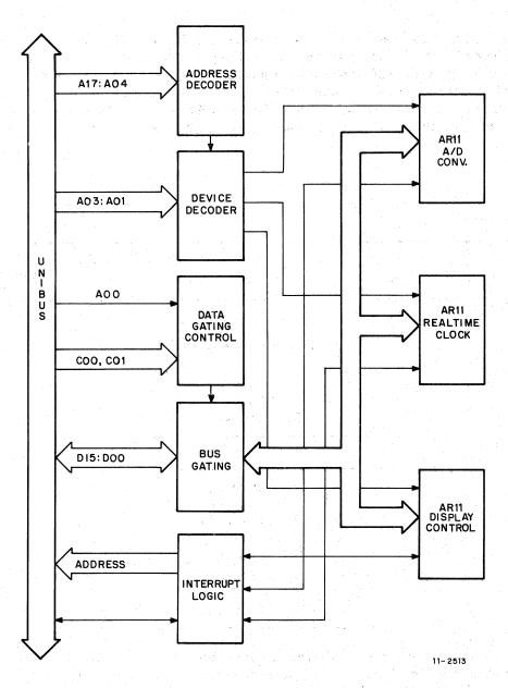
Figure 1-1 AR11 Block Diagram
