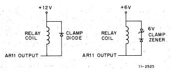
Figure 4-3 Clamping Circuits for Inductive Loads
