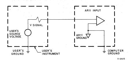
Figure 2-1 AR11 Input Referenced to User's Ground
