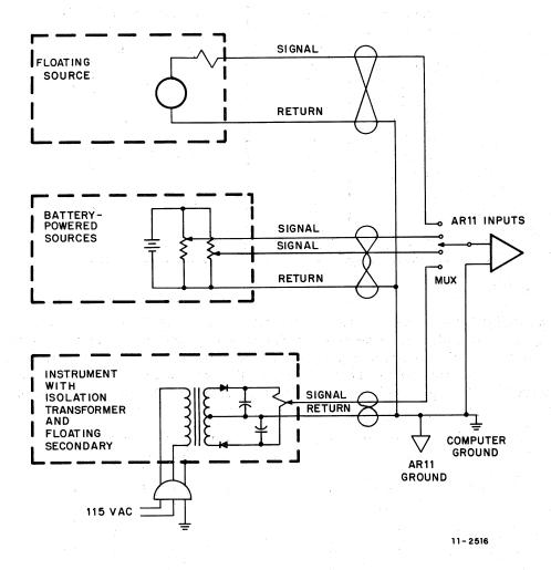
Figure 2-2 Floating AR11 Input Signals
