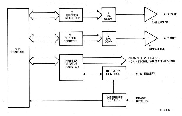
Figure 4-1 Display Control Block Diagram
