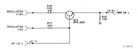
Figure 3-8 PWR OK L Circuit
