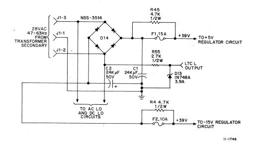
Figure 3-6 Rectifier and LTC L Circuits
