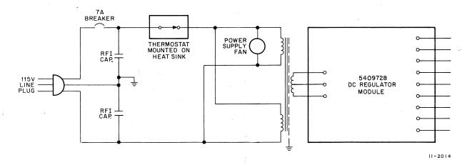
Figure 3-3 115 V Connection, Simplified Schematic Diagram
