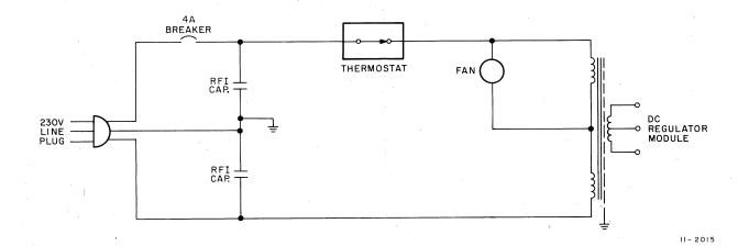
Figure 3-4 230 V Connection, Simplified Schematic Diagram
