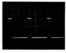
c) Point A, 20A load, 20 μs/div, and 10V/div.
