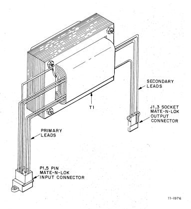
Figure 1-3 Transformer Assembly
