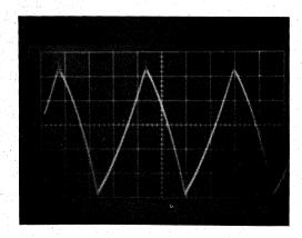
f) Point D, 5A load, 50 μs/div, and 50 mV/div.
