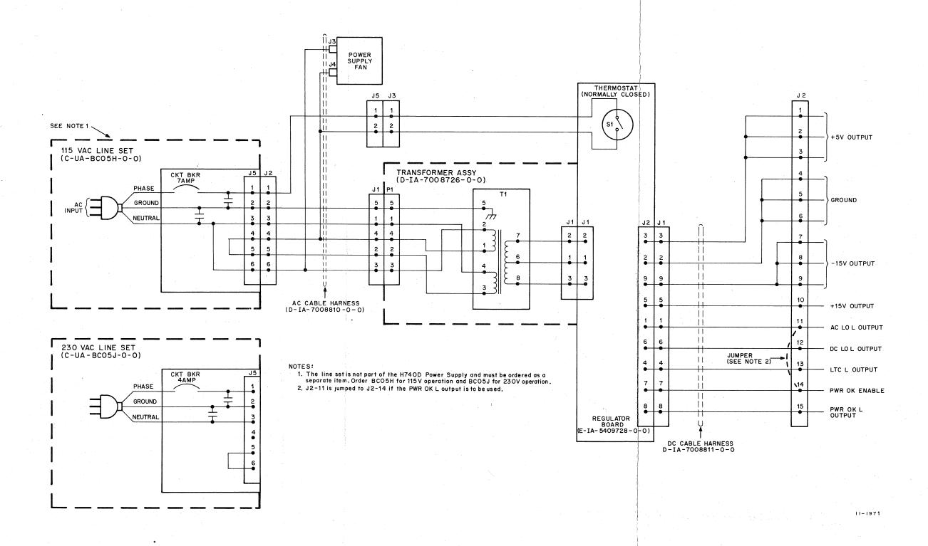
Figure 3-2 H740D Power Supply, Wiring Diagram
