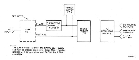
Figure 3-1 Power Supply Block Diagram
