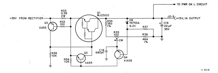
Figure 3-9 +15 V Regulator Circuit
