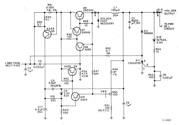
Figure 3-10 +5 V Regulator Circuit
