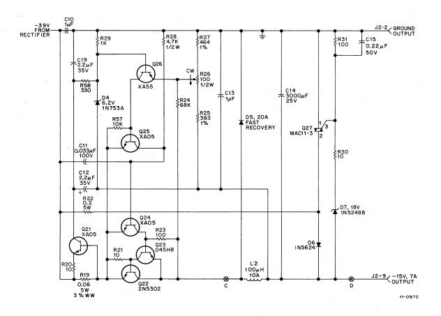
Figure 3-11 -15 V Regulator Circuit
