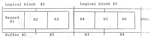
The record length is fixed; the blocking factor is 3. Note that the last portion of the last buffer of each logical block is wasted.
