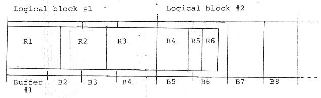
The record length is variable, the blocking factor is 3. The first 3 mecords are the maximum length; the next 3 records are much shorter causing over 2 buffers to be wasted.
