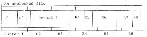
The record length is variable; the blocking factor is Ø
