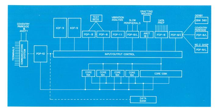
KDF9's, making it possible to increase processor utilization to 70-80 percent. When both KDF9's operate in this manner, their work capacity will be much greater than in their former stand-alone configuration.
